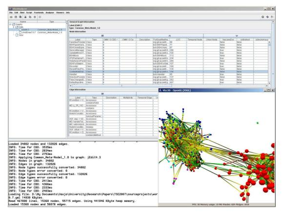
Fig. 3. Example: Metrics analysis and visualization of JEDIT and JHOTDRAW. The VizzAnalyzer (top) shows nodes and edges of JEDIT including some basic information and metrics values (CBC and LOC). Vizz3D (bottom, right) shows a 3D visualization of the call and access structure between classes of JEDIT using a force-based clustering algorithm. Coloring of nodes corresponds to packages.
