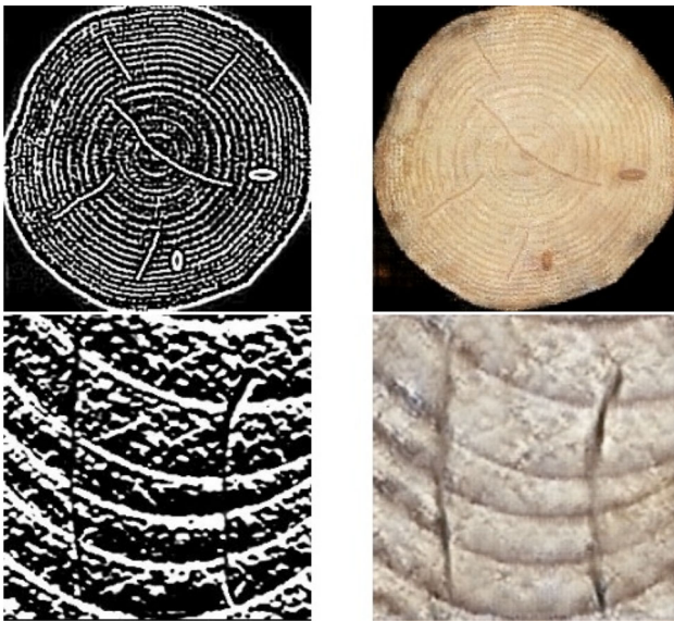
Fig. 7 Examples of added perturbations to the generated images. A perturbations is added to the generated edge map. We add black or white lines to the generated edge maps to represent cracks, and oval structures to represent knots. These representations translate into quite realistic representations of cracks and knots in the generated image
